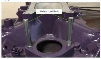
7. Slide the lower plate over the studs.
