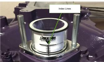
9. Next slide the upper plate over the studs and onto the glass. Don't forget to remove the paper from the seal first.
