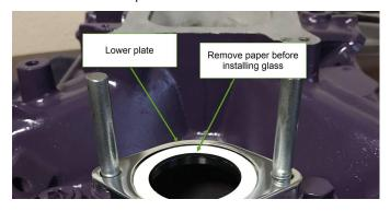
8. Then install the glass making sure the index lines are where you want them. Once you place the glass on the seal you may not be able to move it. The adhesive on the seals is very sticky.
